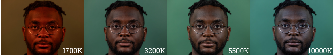
Figure 2.6: This figure displays the range of color temperature settings available on the Nanlite Forza 60c lights in our studio. All images were captured with a 200mm focal length lens and white balance of 5600k. The first image (left) shows a temperature of 1700K (candlelight), the second image represents 3200K (tungsten/incandescent), the third image represents 5500K (daylight), and the fourth image represents 10000K (clear blue sky).
