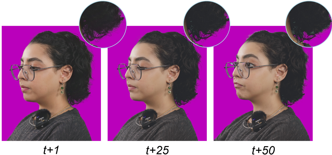
Figure 5.2: Illustration of the drift in accuracy observed in the video matting network starting from the 50th frame.
