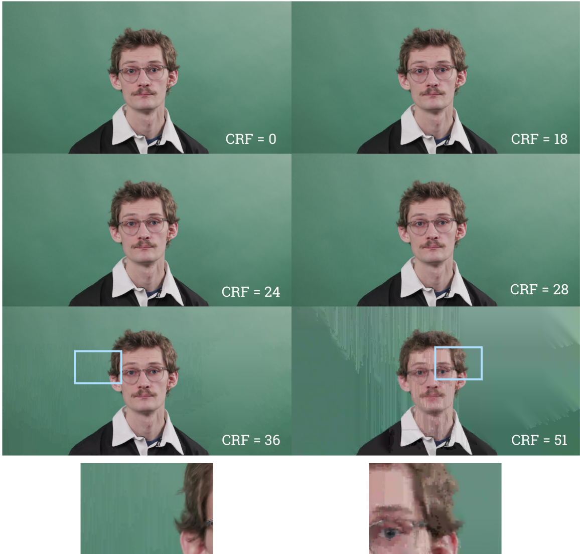
Figure 3.7: Comparison of video quality and file size across different CRF values. As the CRF value approaches 51, compression artifacts become more noticeable.
