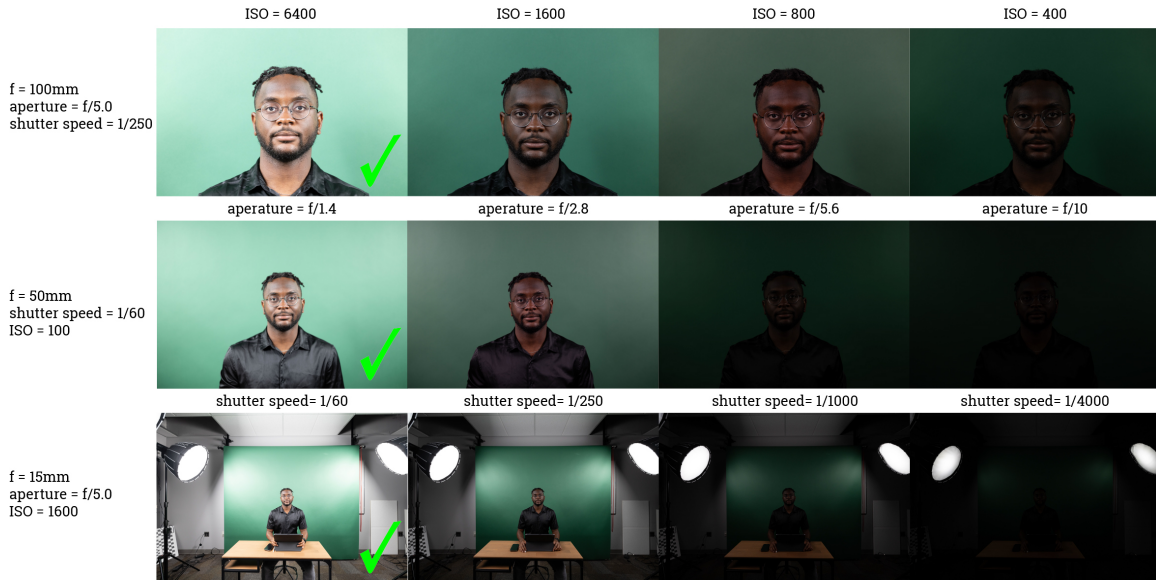
Figure 2.16: This figure demonstrates the effects of varying ISO, aperture, and shutter speed on image exposure. Each row represents images captured with a fixed focal length and a fixed pair of two exposure settings, while the third setting varies across the columns. The first row shows the impact of changing ISO, the second row, aperture, and the third row, shutter speed.
