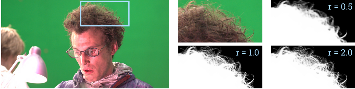
Figure 4.15: Comparison of alpha mattes generated at different inference resolutions: half the original resolution, the original resolution, and twice the original resolution, highlighting the improvement in detail preservation and edge precision at higher resolutions.
